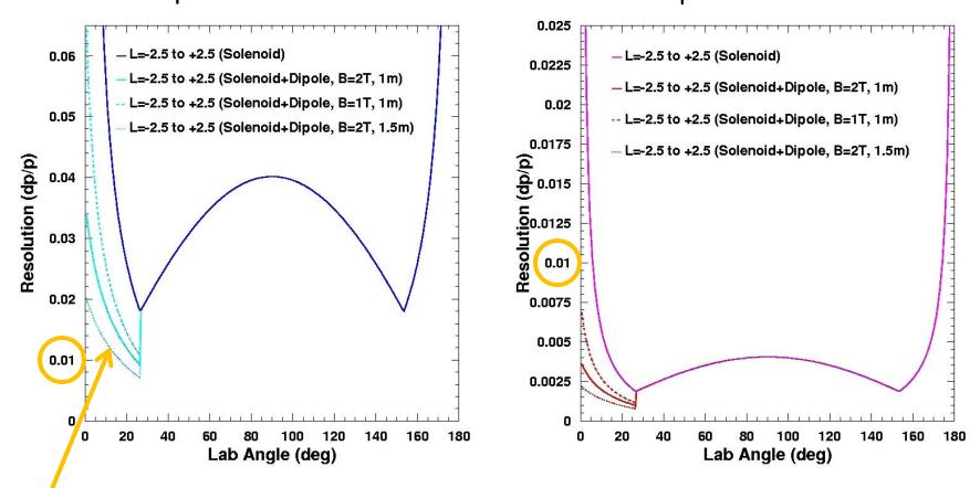
As expected, substantially improves resolutions at small angles
