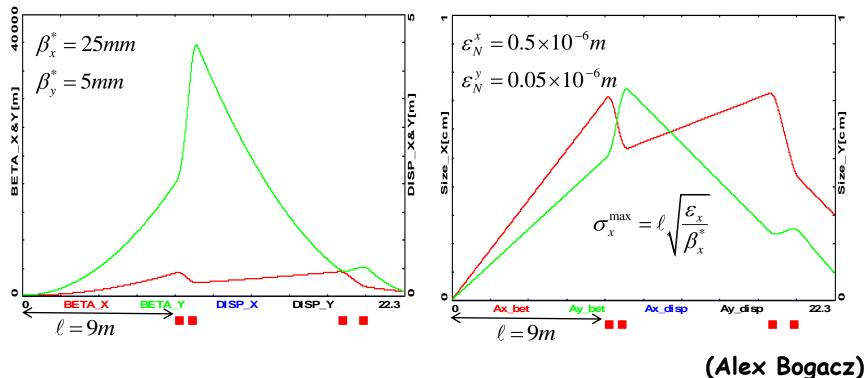
Manageable beam sizes at the FF quads ( $\sigma_{RMS} \sim 5 \text{ mm}$ )
