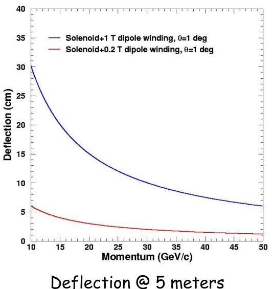
• 0.5-1 Tm dipole component, or 2 Tm separate dipole sufficient on hadron side to peel the charged particles away from beam line and allow for tagging/vetoing? Need to fold in map of angle vs. momentum of particles of interest to better constrain. • Of course, such options also need to be checked
