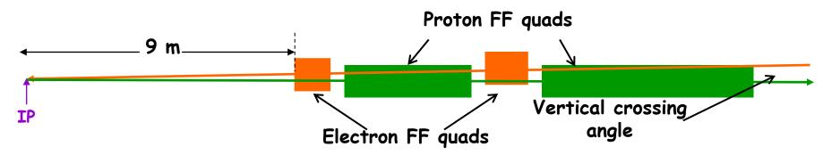
If ELIC w. 8 m IR space  $\rightarrow$  Proton FF quads of 1.8 (3.0) m with 20.8 (12.0) kG/cm
