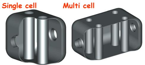
(top) Multi-cell TM110 and Loaded Structure of Crabbing Cavity (JLab/Cockcroft/Lancaster)
